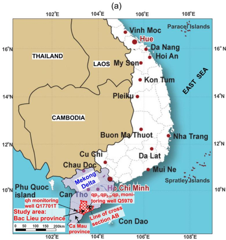
**Fig. 1.** Map of Southern Vietnam showing the study area (Bac Lieu province) within the Mekong delta including groundwater monitoring wells and hydrogeological cross-section AB location illustrated (at the top). Hydrogeological cross-section along line AB (below). The bore-holes (wells), their ID and depth indicated as well as semi-permeable sediment layer (quaternary, yellow colored), aquifers (blue colored) and fault position provided.
