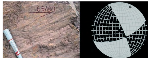
Fig. 4. The normal left fault with orientation 065/80 and striation pitch angle 250 at the survey location TY-LS-13. The analytical result determined the stress state: Sigma 1: 290/24; Sigma 2: 134/63; Sigma 3: 024/09.
