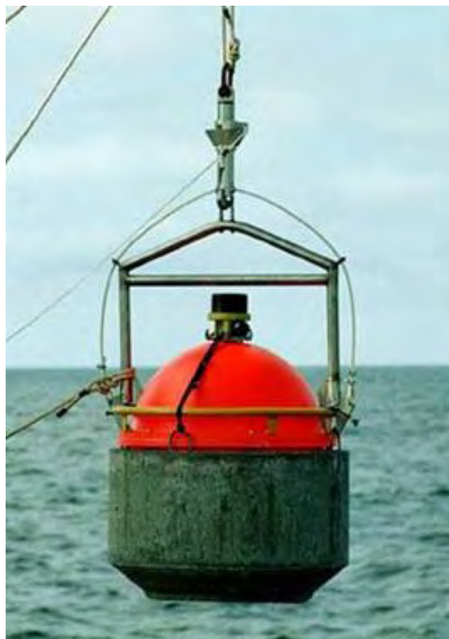
Fig. 4. General view of the self-floating ABSS prepared to installation.
