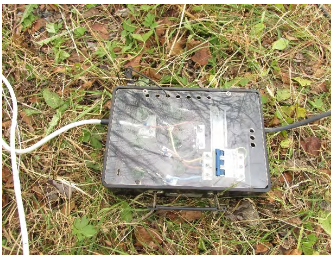
Fig. 4. The exterior of three-phase rectifier – a current source in electrical soundings of 7–10 November 2022 (left). Recording of 13 A current on the voltmeter at the moment of a separate pulse (right).
